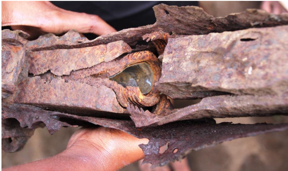
Breech of the apparent .50 cal. machine gun located near and likely from the Corsair wreck, The shell in the breech exploded when the gun was put in a fire in March 2013 – who says American made products don't last!
