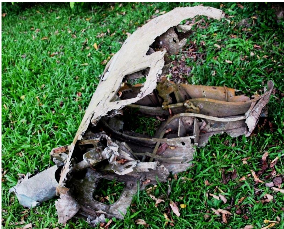
Western-most wreck part in Nanako, moved from the original wreck site to the front yard of the Toa Palms Bungalow. This wreckage had a number which matched the F4U-1 parts manual. This is the tail section of the plane, with the upper portion on the left. The protruding part at left led up to the tail rudder.
