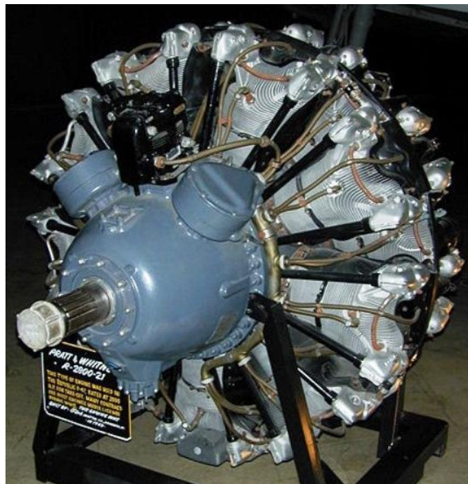
The front of a Pratt & Whitney R-2800 engine, in slightly better condition than the Nanako engine (from Wikipedia)
