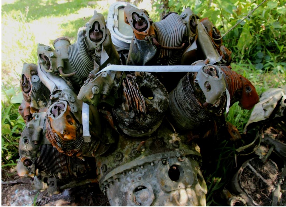
Top of engine with tape measure, showing double row of cylinders
