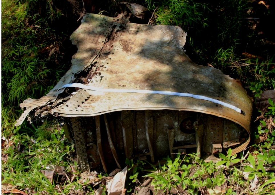
Second easternmost plane wreck part, with one yard tape measure; This is the starboard inner wing, according to Bob Jarrett of the Classic Jets Fighter Museum
