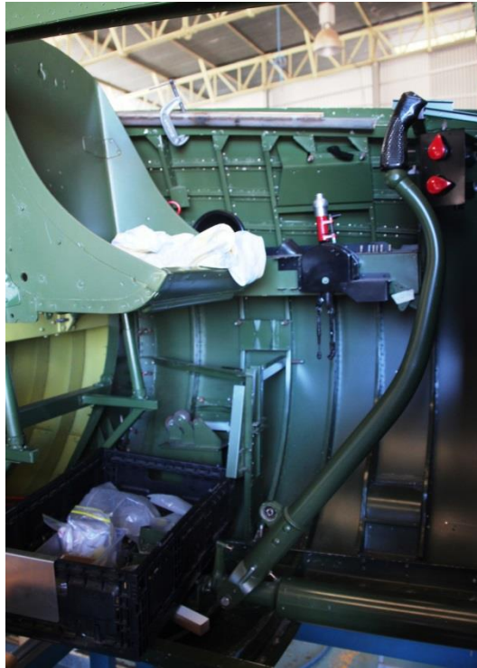
Partially restored interior of the Corsair, showing the “stick” at right and pilot’s seat at left
