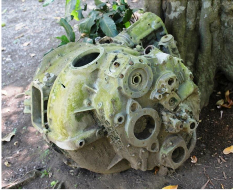
Supercharger of the plane in Nanako, the most westerly part in original wreck area
