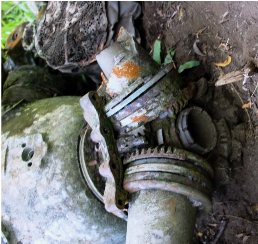
Three bladed-propeller hub on Nanako plane
