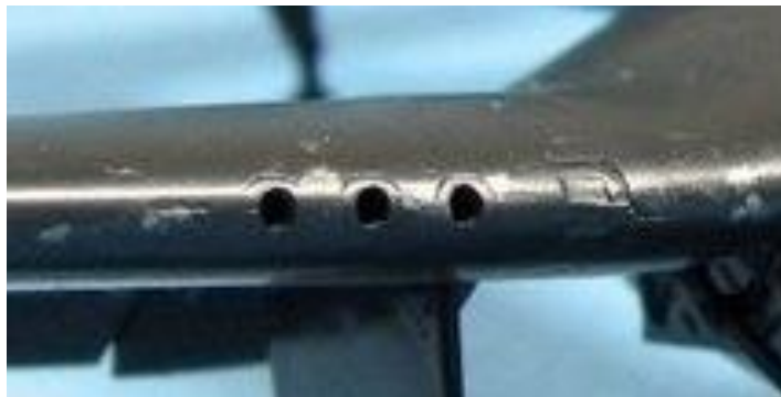
Machine gun ports on an F4U-1
