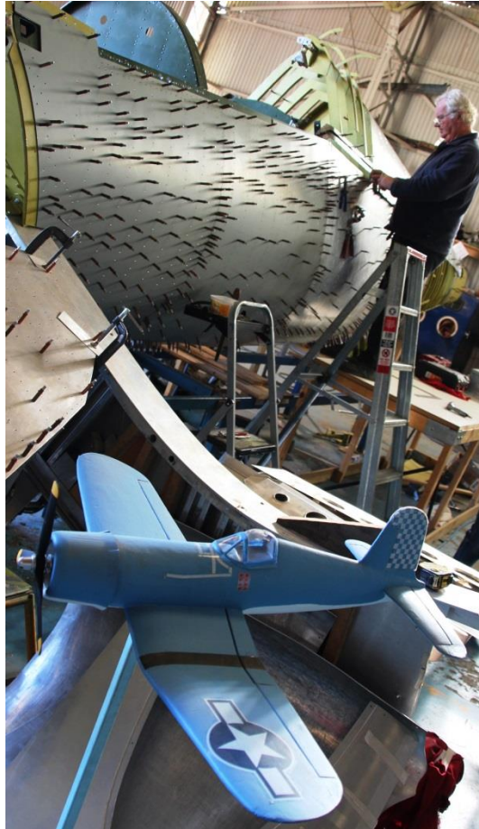
Model of the Corsair in foreground and workman restoring the fuselage in the background. The numerous pins hold the skin in place until rivets can be installed.
