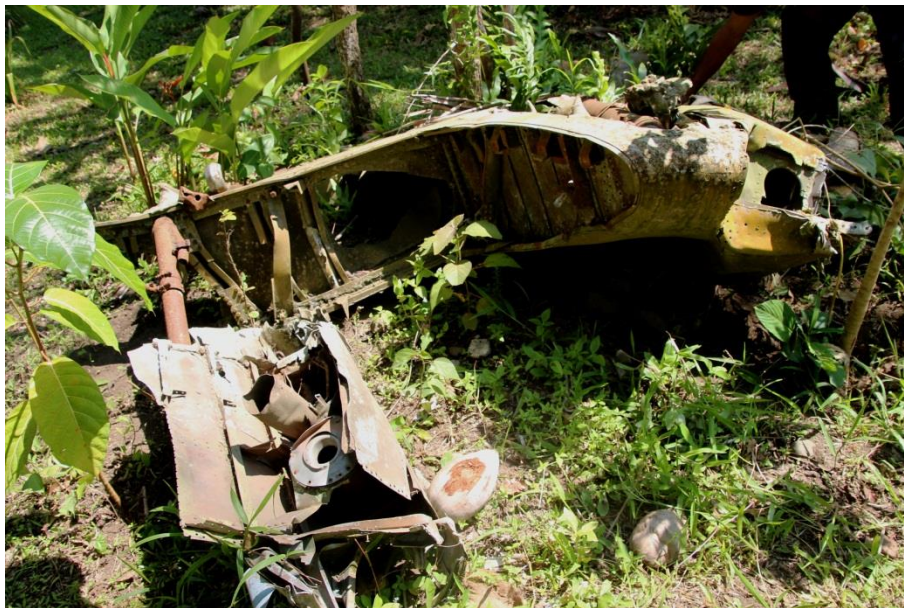
Easternmost portion of Nanako wreck, including the machine gun support ring, seen in the lower left as a round ring with a round hole in it. This part had a number matching the parts manual.
