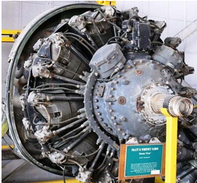
Rear of Pratt & Whitney R-2800 engine (from Wikipedia)
