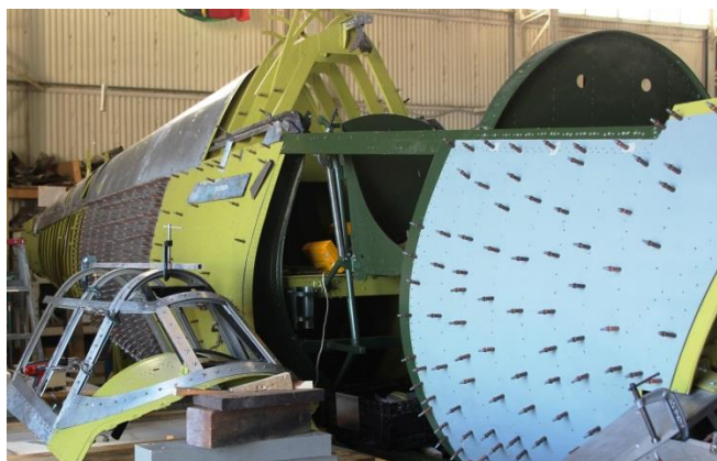
Fuselage of the Corsair, with pilot’s seat in center and separate canopy at lower left. Parts from Nanako are behind and to the left of the pilot’s seat.
